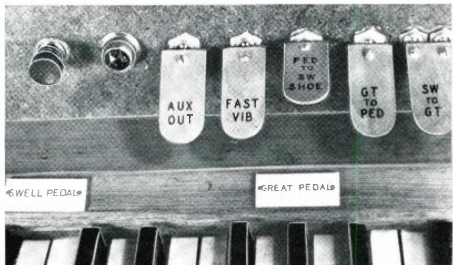
Fig. 35. The coupler panel. It is located on front panel just above swell manual.
