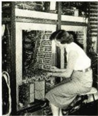
COVER PHOTO: Technician works on the analogue computer console at Convair's Computer Facility in San Diego. This million dollar unit solves aircraft flight problems. For full operational details, see story on page 61. (Ektachrome by Roger W. Jett)
