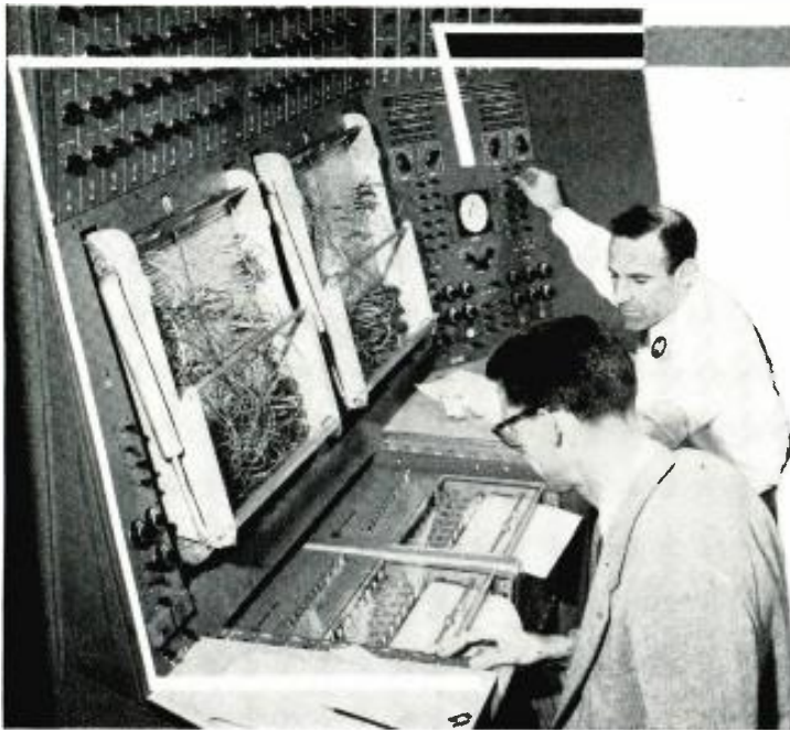
Fig. 1. The "Convair" analogue computer in operation. Two problem patchboard stations in normal operating position are shown in one-half section of the dual computer console. In the foreground the engineer checks mobile recorder unit which draws graphs that are the solutions to the problems on the computer. The resistance and capacitance decade boxes are shown at top.
