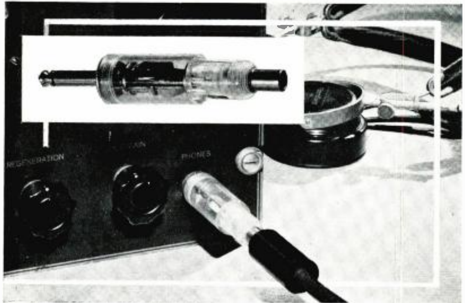
Fig. 1. The plug in use in receiver setup. (Inset) Close-up of phone-plug amplifier.
